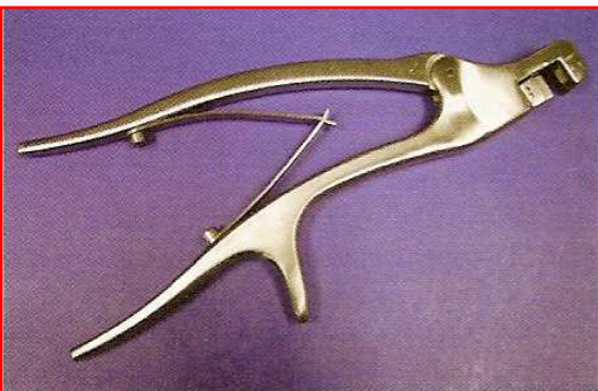
Figure 3 | Prototype plate bender, used to contour plates for spinal surgery, built by DePuy using a laser-sintering system.
