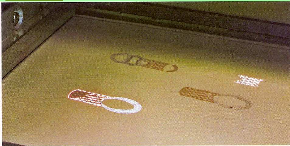
Figure 1 | Laser sintering in action. A laser beam melts a layer of metal powder which then solidifies. By repeating the process a three-dimensional part can be made.
